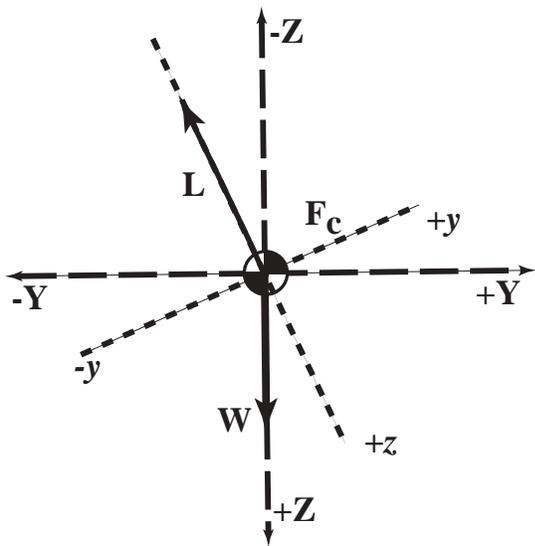
**Figure 1.** Forces in the  $yz$  plane acting on an aircraft in a steady state gliding turn.
