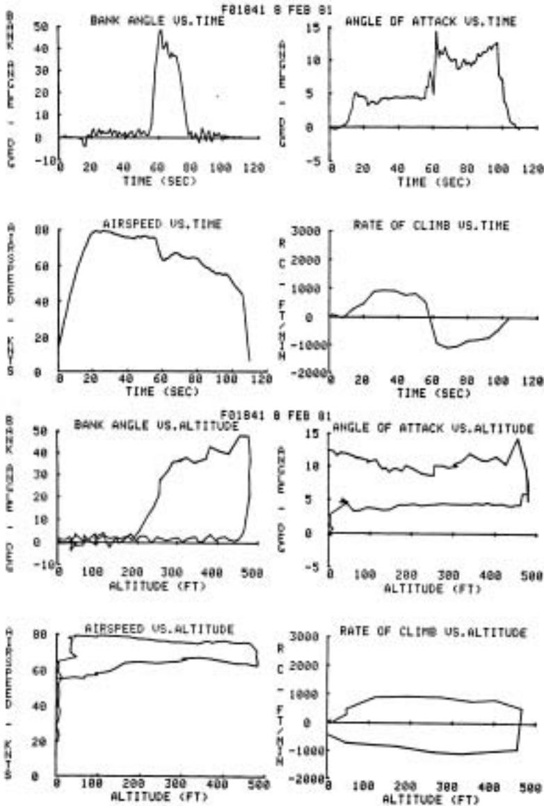
Figure 11b. Graphic output of the flight parameters from a successful test flight.
